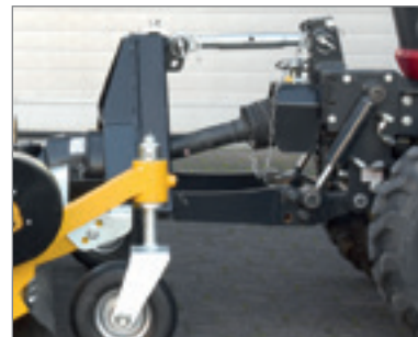
With mounting parts for Kubota, John Deere, Iseki, Shibaura and coupling triangle. Other models on request.
