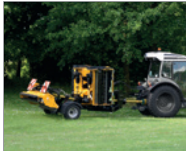
Small transport dimensions and a chassis design with wide tyres guarantee a smooth ride that protects the soil.
