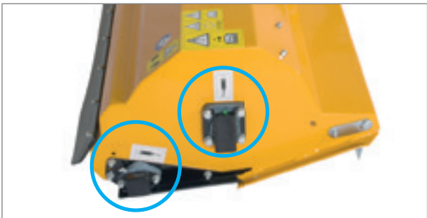
Easily accessible bearing points for quick maintenance.
