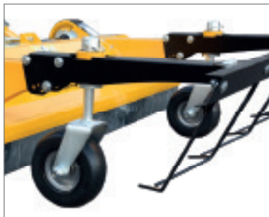
Vertically adjustable support wheels, 360-degree swivelling
