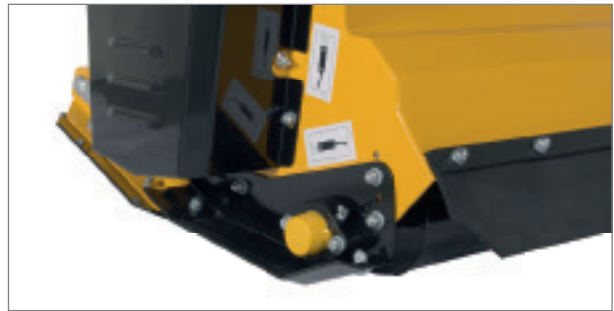
Finally graduated, adjustable support roller for depth guidance.
