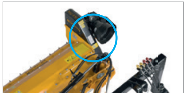
V-belt tension is always visible: V-belt protection with inspection opening.
